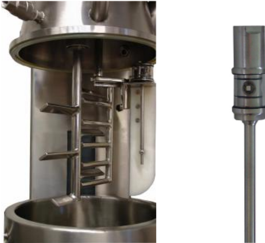
Figure 4: Temperature Measuring System with Infrared Transmittance a) (on the left) installed in the Planetary Mixer b) (on the right) Sensor
